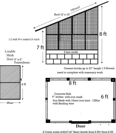
4 Coner poles with(4"x4" Bars) length 2nos 9.5ft+2nos 8.5ft ( 2 Bars of 4"x4" 2mm can be utilised)
